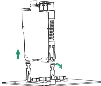
Pull the slot of the backplans outward, and remove the apparatus as arrow shows .
